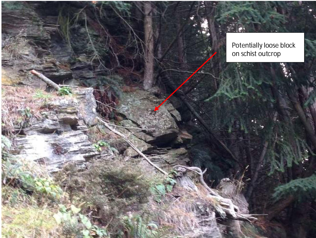
Photograph 7 Typical Area Type B, low bluffs and rock exposures with potentially unstable blocks present in the surface.
