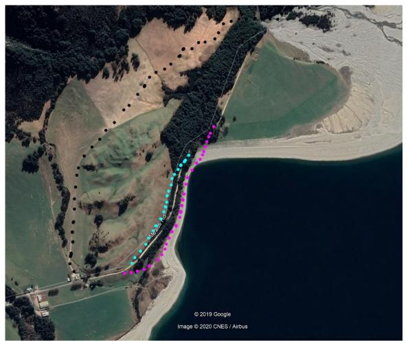
Figure 4 Alternative routes to avoid the slip. High level shown green, beach level shown purple, and longer route shown black
