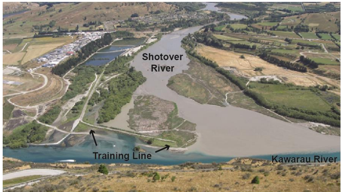
Figure 4. View up the Shotover Delta during high flows in 2013. The training line visible on lower left of image directs the turbid water of the Shotover River to the right to meet the clear water of the Kawarau River at an oblique angle. Kawarau River flows left to right.
