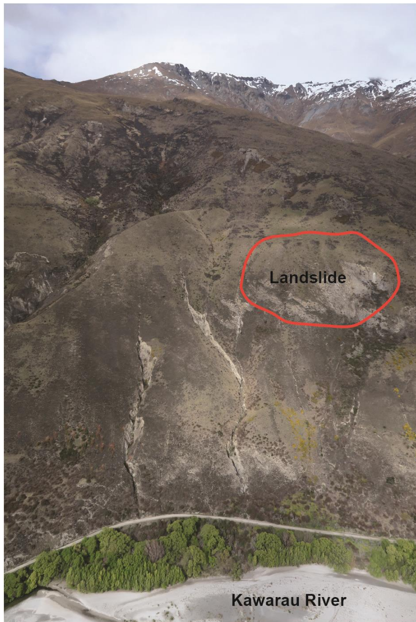
Figure 8. Incipient bedrock landslide above the Kawarau River approximately 1.6km upstream of the Arrow River confluence. This landslide has sufficient volume to dam the river if it failed as one mass. The landslide is monitored by ORC.
