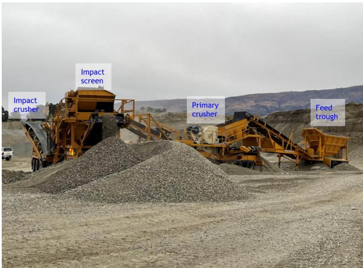
Figure 3. Components of mobile crusher.
