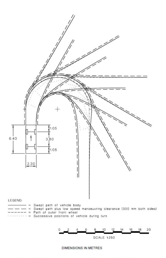
Turning Path Template - Small Rigid Vehicle
