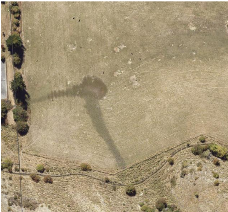
Figure 6.1. Seepage and ponding, in the area of proposed Lot 2.
