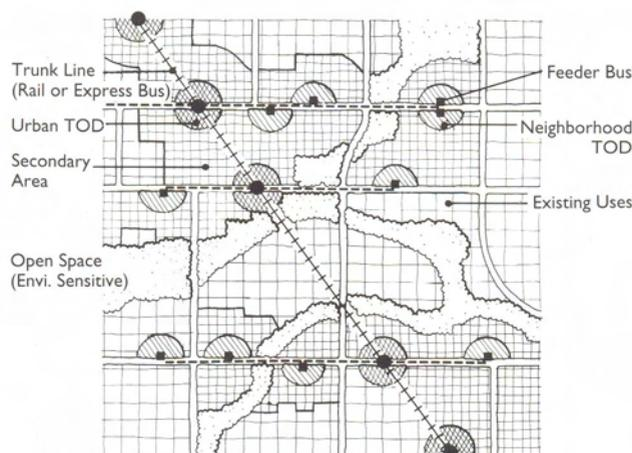
The trunk line network represents the region's express transit system. It typically consists of either light rail, heavy rail, or express bus service, with at least a 15-minute frequency of service and a dedicated right-of-way. Providing a dedicated right-of-way, whether fixed rail or HOV lanes, serves two important purposes: 1) it ensures expedited and free-flow transit travel; and 2) it represents a long-term transit commitment that allows developers to make similar investments.
