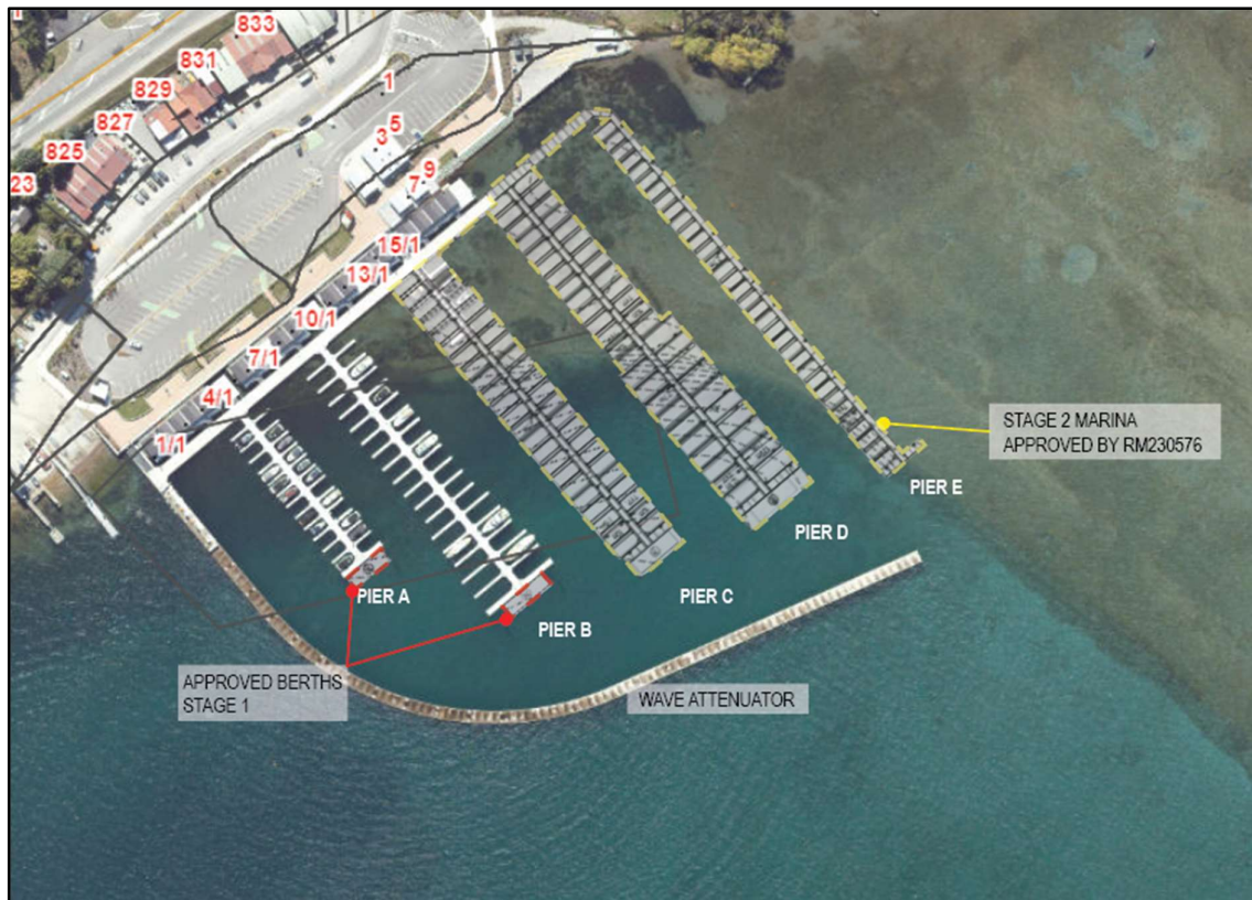
Figure 1: Aerial imagery of the constructed marina (Stage 1), car park and buildings, and overlay of Stage 2 marina plans (approved and to be constructed)
