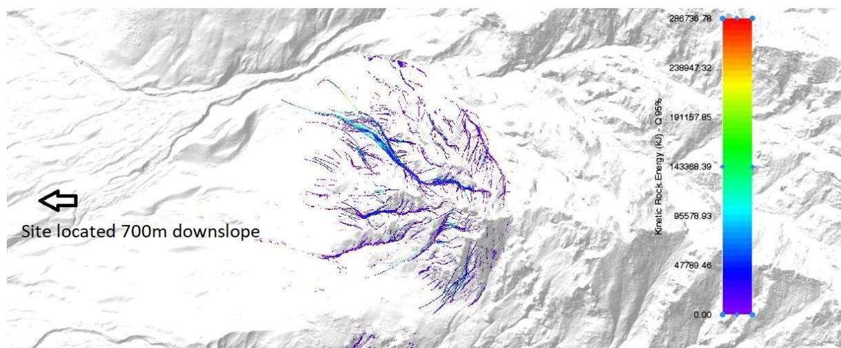
Figure 2: Screen shot showing theoretical trajectories of all modelled rock falls from an area release type (Remarkable Bluffs) with trees not present on the slopes beneath. The site is located downslope and is not shown.
