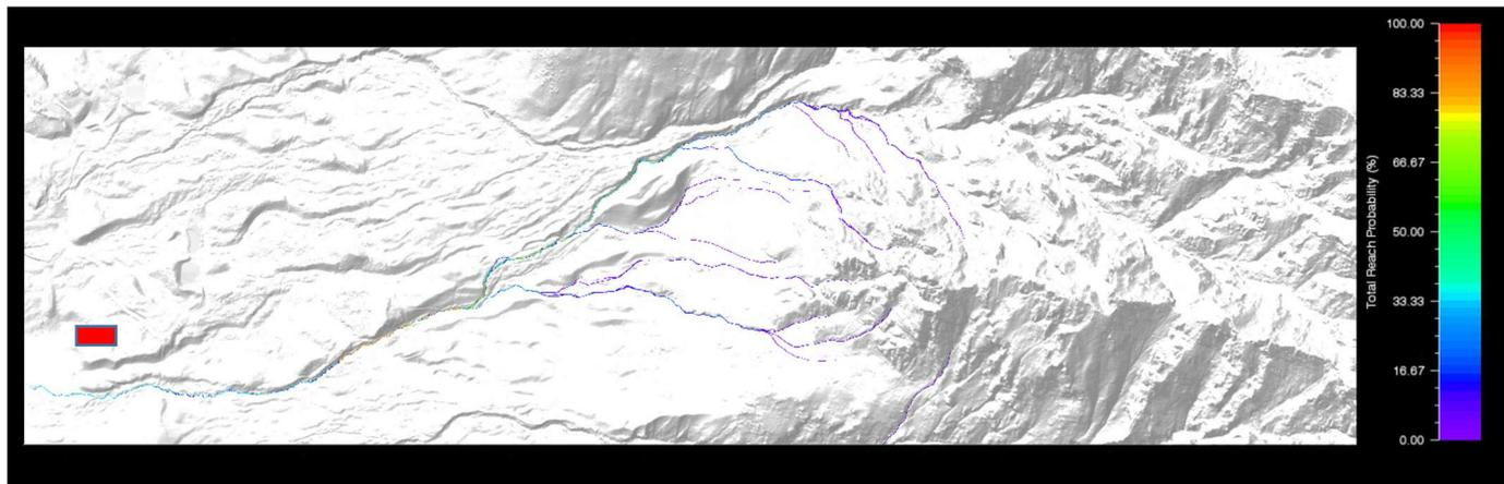
**Figure 3: Screen shot showing the probability that a modelled rockfall will reach a given cell within the model (total reach probability) of all modelled rock falls from an area release type (Remarkable Bluffs) with trees not present on the slopes beneath. The site boundary of the site boundary is shown in red.**
