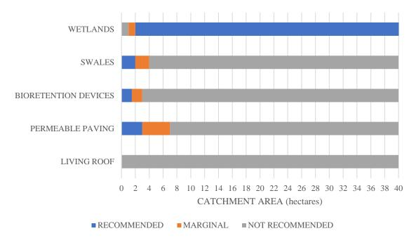
*Figure 5.13 – Recommended catchment areas for different water quality treatment devices. Figure reproduced from Auckland Regional Council Technical Publication 10 (May 2003).*
