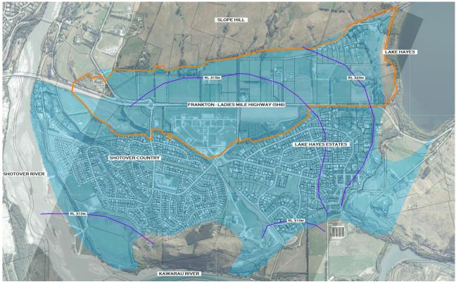
*Figure 5.4 – Windemeer Aquifer extents and levels. Figure reproduced from Otago Regional Council Investigation into the Wakatipu Basin Aquifers (July 2014).*
