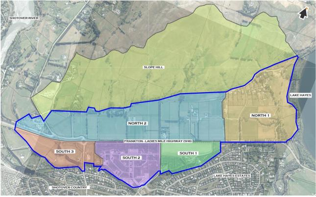
Figure 3.1 – Proposed masterplan stormwater management catchment delineation.
