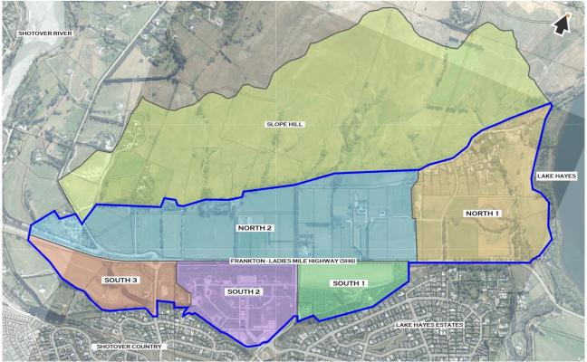
Figure 5.6 – Proposed masterplan stormwater management catchment delineation.
