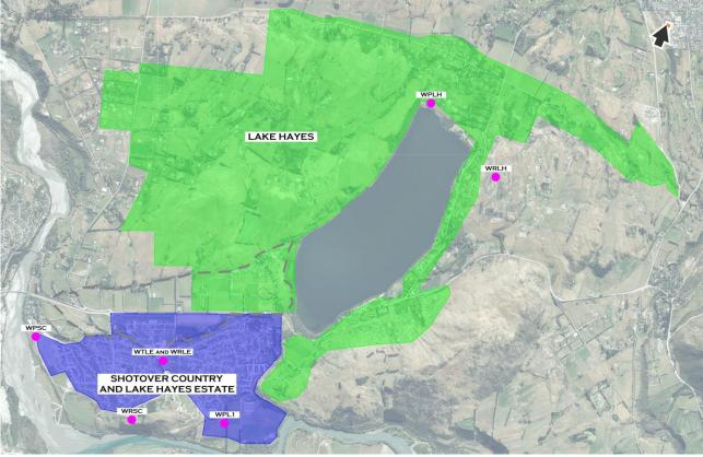
*Figure 7.2 – Indicative existing public water supply service area including the location of the pump stations, treatment plants, and reservoirs.*
