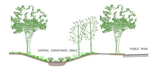
Figure 5.10 – Slope Hill central conveyance swale.
