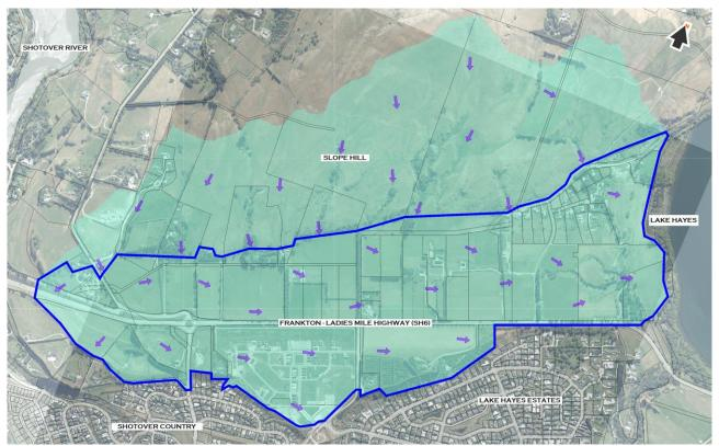
Figure 5.5 – Proposed masterplan catchment extent and likely surface water flow direction.
