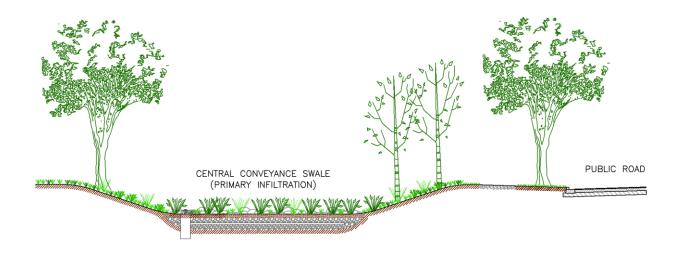
Figure 5.11 – Slope Hill central conveyance swale infiltration section.
