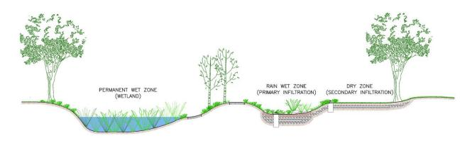
Figure 5.9 – Stormwater management area zone layout.
