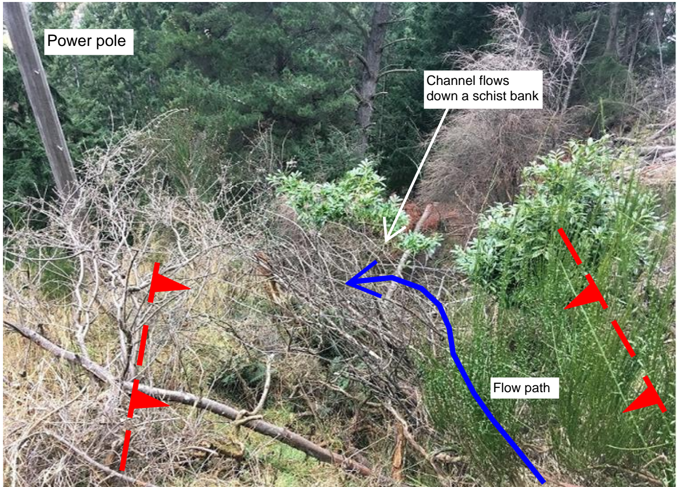
Photograph 12b. DL2 flow channel Section 12b. Channel bed is heavily vegetated in grass, fern and broom scrub.
