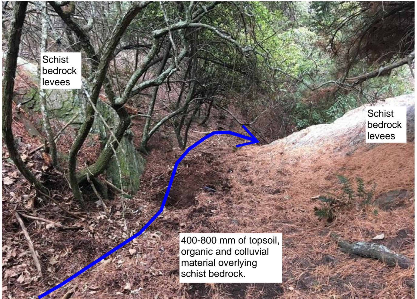
Photograph 11b. DL2 flow channel Section 11b. No evidence of recent scour erosion.
