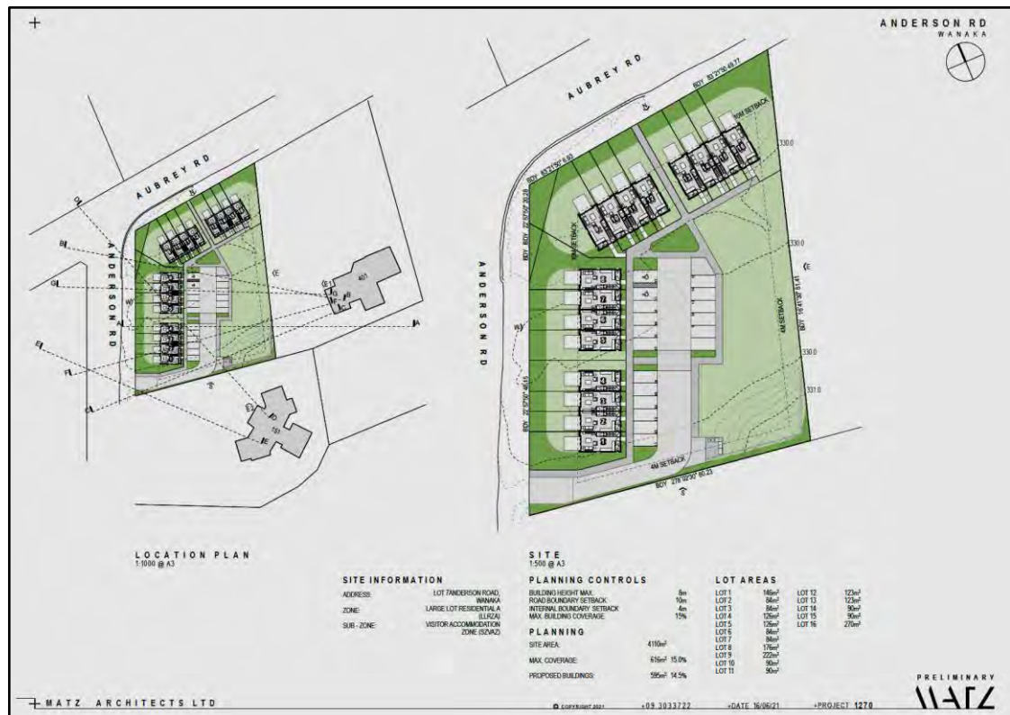
Figure 8: Example of a complying proposal at 14.5% site coverage (refer to Appendix 2A).
