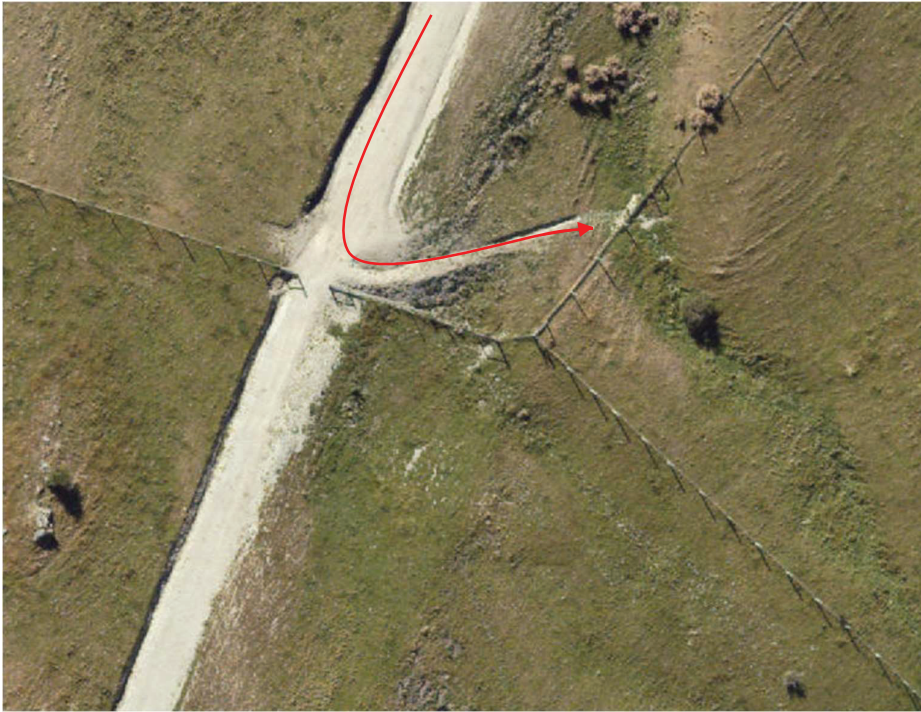
Figure 5 Diversion drain into existing overland flow path
