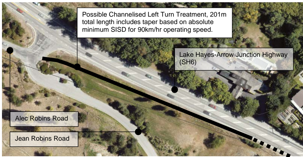
Figure A2: Possible Channelised Left Turn Treatment, SH6 to Alec Robins Road
