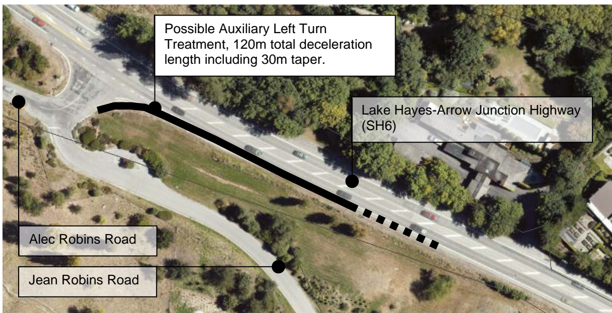
Figure A2: Possible Auxiliary Left Turn Treatment, SH6 to Alec Robins Road
