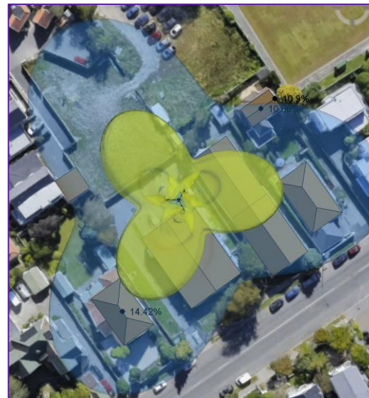
An example of RF Lobes – Plan view
