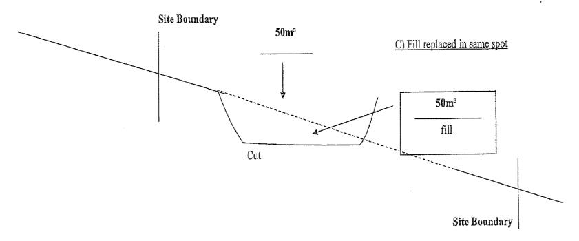
6. The distance between the boundary and the cut or fill shall be at the top of the cut batter/slope/face or to the toe of the fill batter/slope/face (as below).
