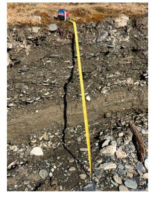
Photo 3: Observed cut slope showing alluvial fan deposits consisting of gravels, sands and silts
