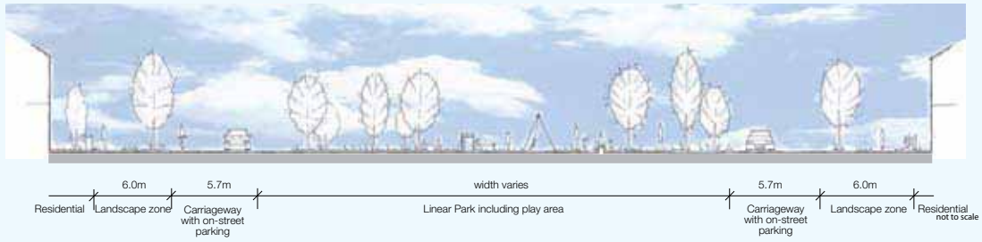
Typical Section F - Linear Park (width varies)
