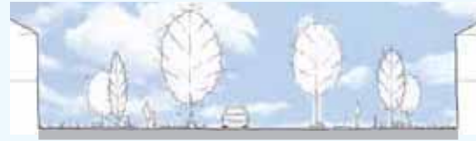
Residential | Landscape zone with informal footpath (5.15m) | Carriageway with on-street parking (5.7m) | Landscape zone with informal footpath (5.15m) | Residential not to scale
