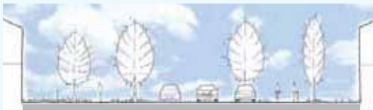
Residential | Landscape zone with tree planting, off-street parking and shared cycle/footpath (7.5m) | Carriageway (7.0m) | Landscape zone with tree planting, off-street parking and shared cycle/footpath (7.5m) | Residential not to scale
