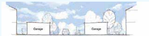
Private Courtyard | Garage Setback (2.0m) | Carriageway (4.0-5.0m) | Garage Setback (2.0m) | Private Courtyard not to scale
