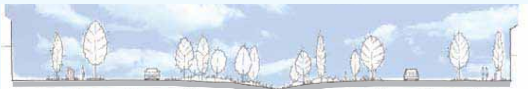
Employment Land | Landscape zone (6.5m) | Carriageway (7.0m) | Landscape buffer (width varies) | Swale (Approx. 15m) | Carriageway with on-street parking (5.7m) | Landscape zone (6.0m) | Residential not to scale
