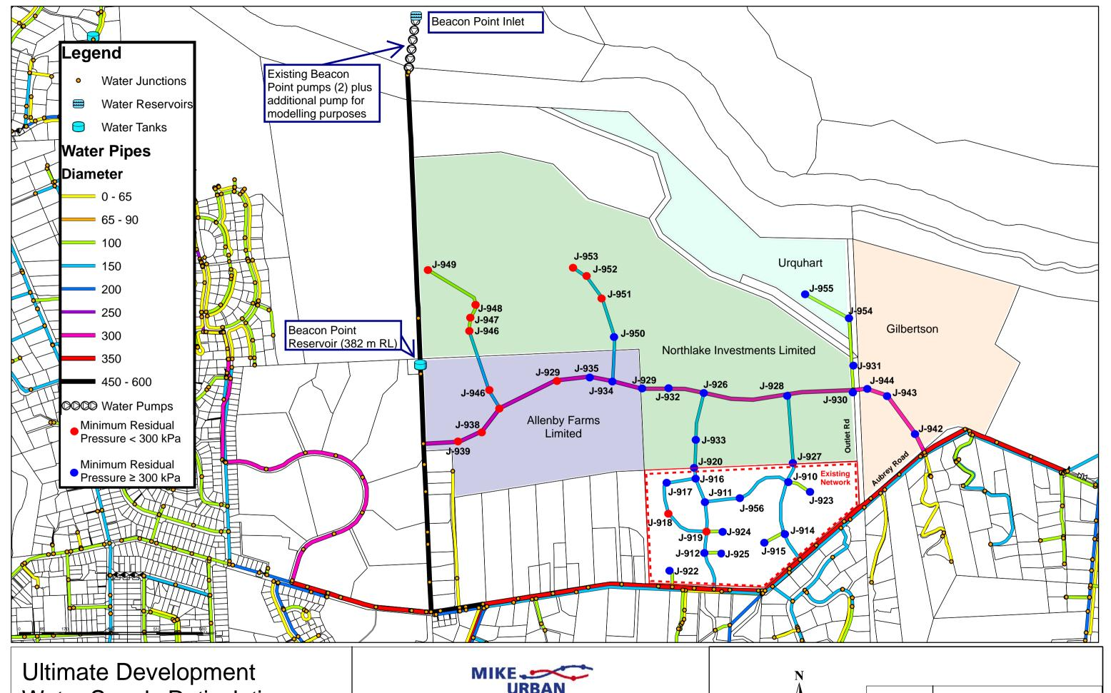
Water Supply Reticulation - with additional inlet pump
