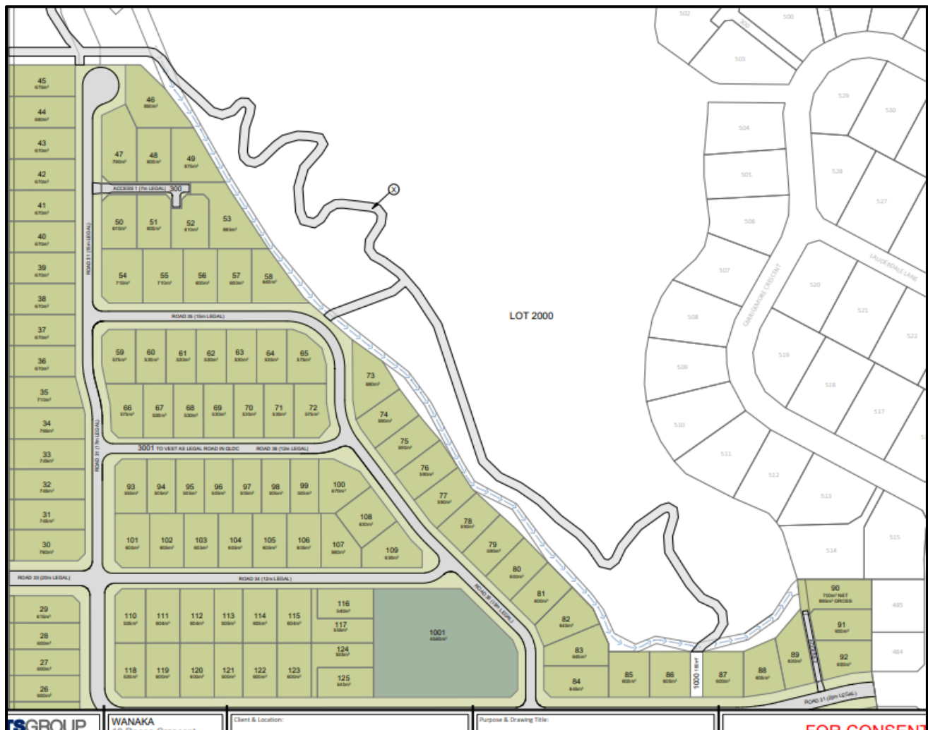
Figure 5: Scheme plan for RM240663 including the pedestrian/cycle trail, that is to be constructed prior to s224c of the final stage of the development.
