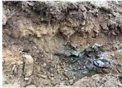
Excavation measures ~3 m x 1.5 m. Bedrock and groundwater was not encountered LOGGED BY: DATE: 16-May-22 METHOD: 18T excavator
