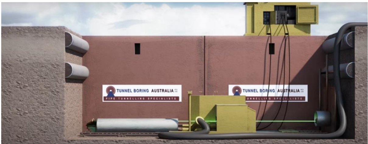
Figure 3: Launch pit, AXIS machine and vacuum head
