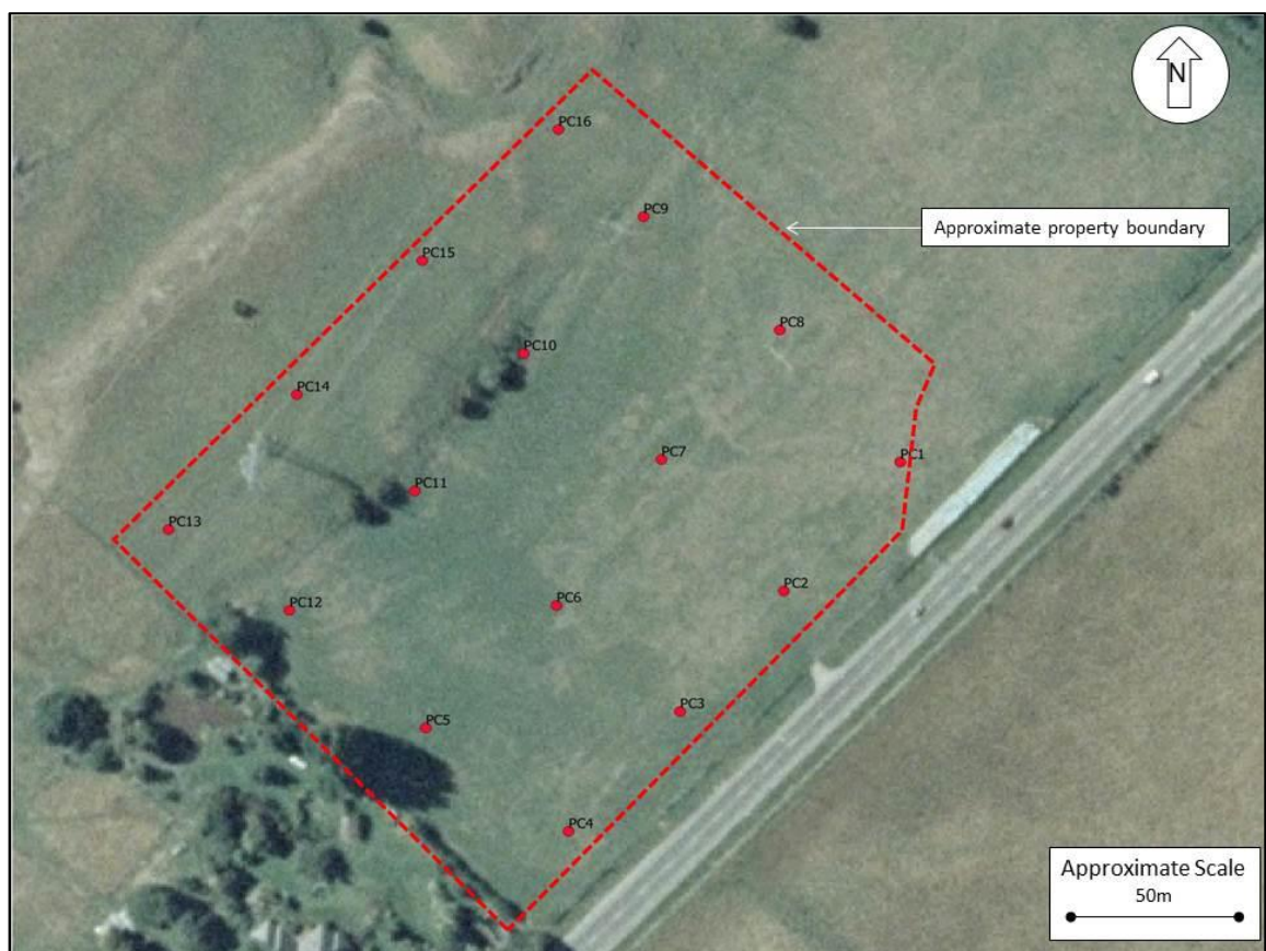
Figure 4: Soil sample location plan.
