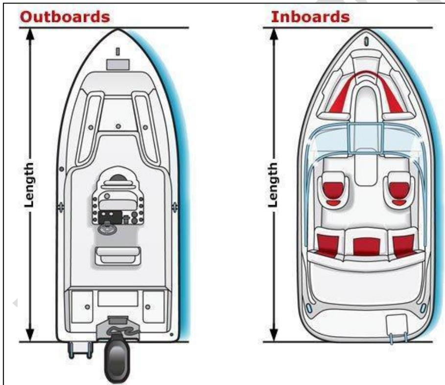
Figure 2 – guide to measuring the length overall of a yacht
