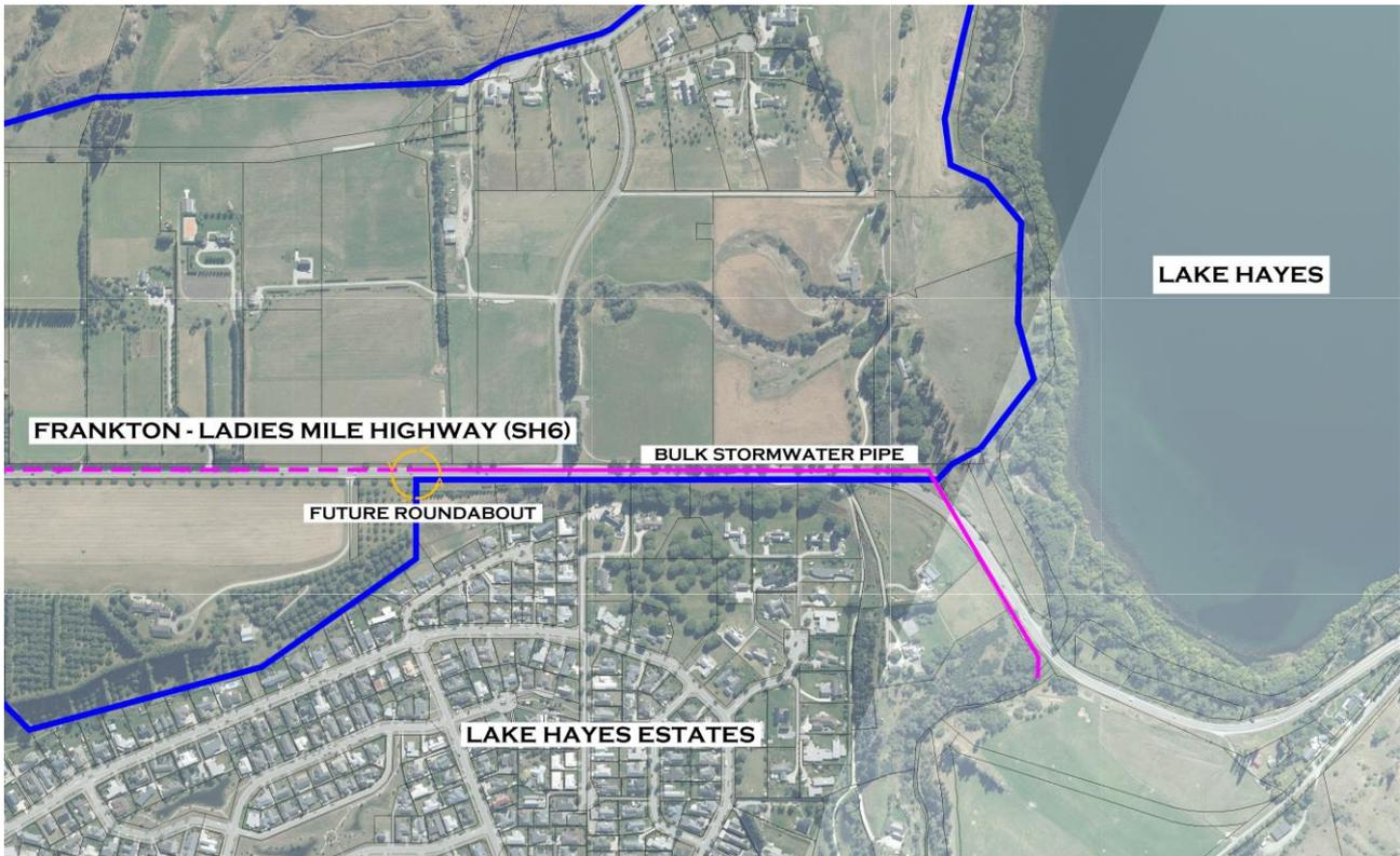
Figure 5.12 – Indicative bulk stormwater pipe route.
