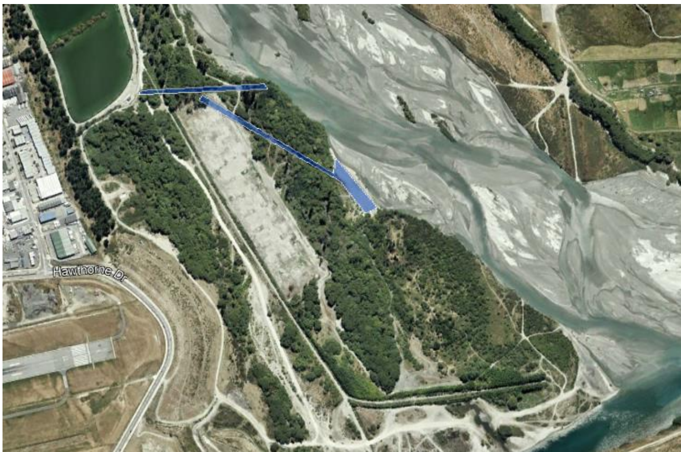
Figure 10 Option 4a, Previous discharge channel indicated in the diagram (blue highlight)
