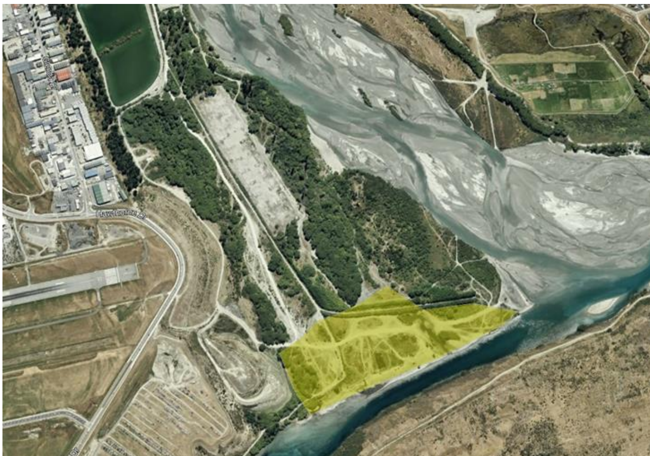
Figure 3 Option 1a Infiltration Basin in the Shotover Delta - indicative site area (yellow highlight)
