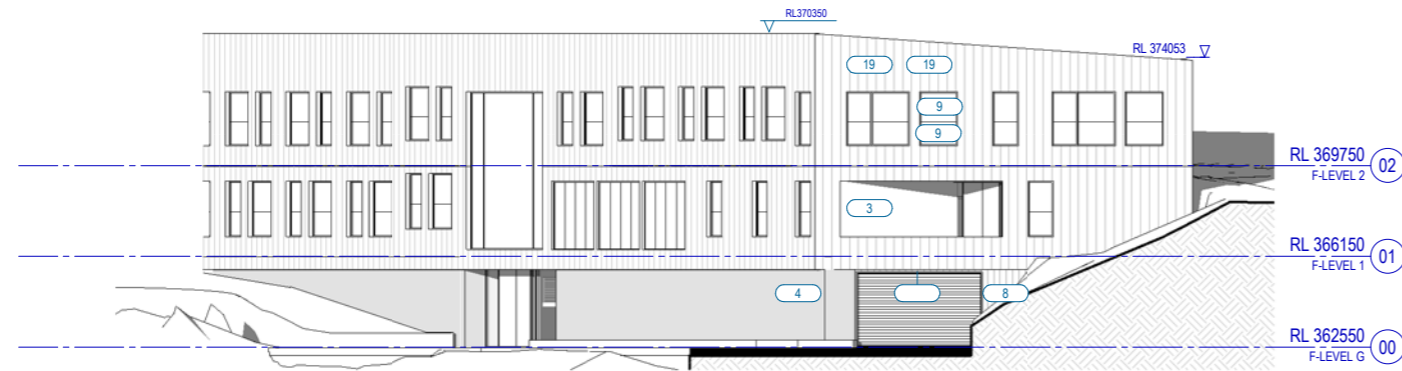
1 F-SOUTH ELEVATION SCALE 1 : 150
