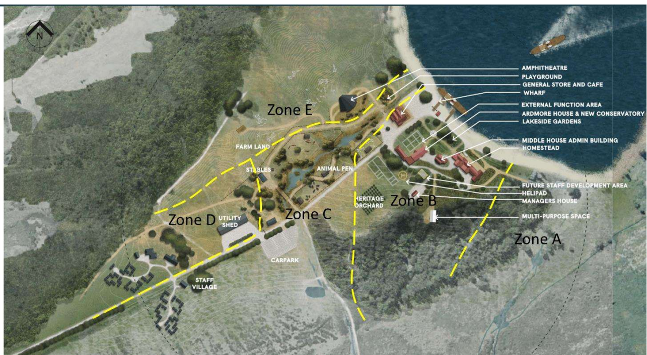
Figure 5: Plan of WPHCF showing key elements of the site development and five zones inferred to have similar lives risk levels. Base image after Beca (2017).
