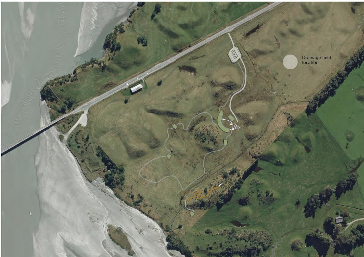
A septic tank system is provided for the 4 toilets located in the nursery area, with black and grey water pumped to a drainage field located over 50 metres from any wetland or waterbody (shown shaded white).
