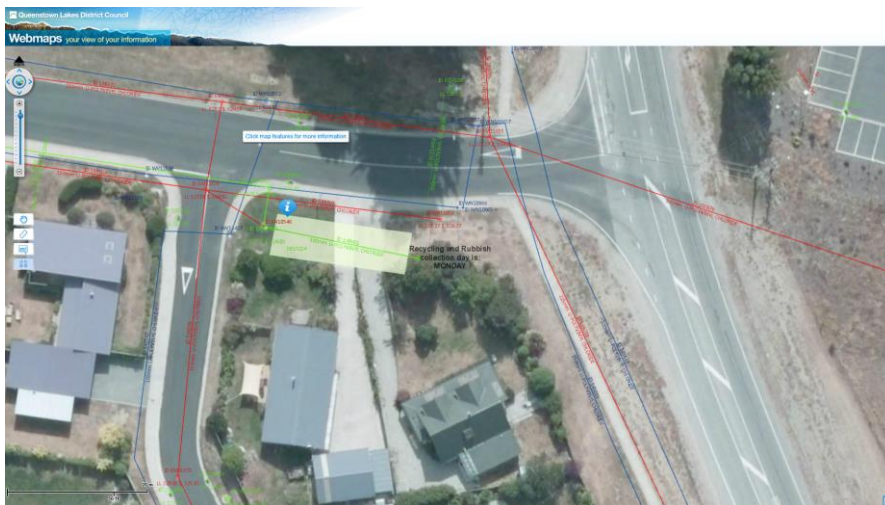
Figure 1 – Subject Site and Existing Services (Soak Pit) Shown Green. Source – QLDC Website 05.03.15
