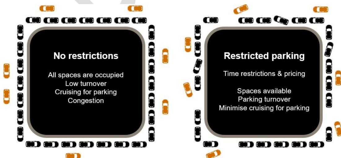
Figure 3: Impact of parking on circulation and congestion
