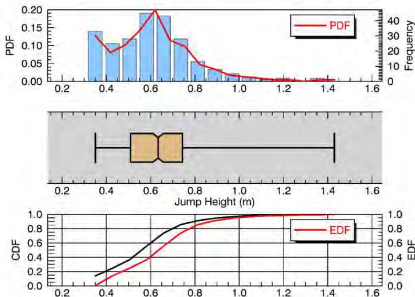
Figure C 3 - Barrier plot showing bounce heights of modelled rockfall trajectories intersecting the proposed location of the rockfall fence on the hillslope to the true right of Brewery Creek (drawing 3209881-C001).
