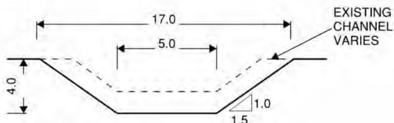
Figure A2 - Brewery Creek channel (modification to existing channel)
