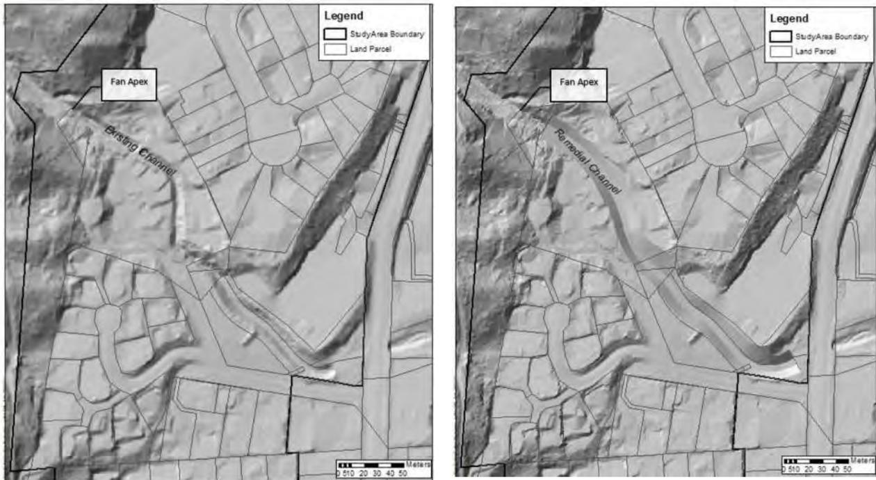
Comparison of the morphology of the existing Brewery Creek channel (left) and the proposed modified channel (right).
