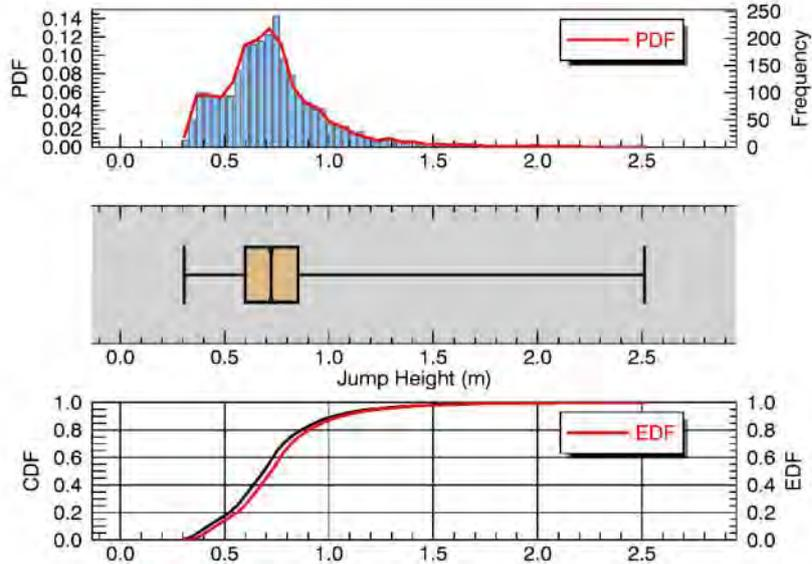
Figure C 5 - Barrier plot showing bounce heights of modelled rockfall trajectories intersecting the proposed location of the rockfall fence on the hillslope to the true left of Reavers fan (drawing 3209881-C002).
