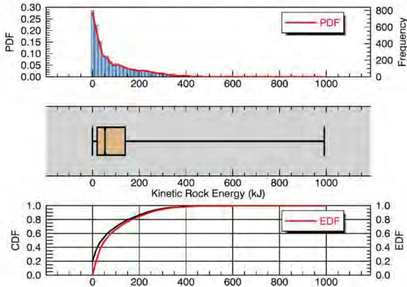
Figure C 8 - Barrier plot showing kinetic energy of modelled rockfall trajectories intersecting the proposed location of the rockfall fence on the hillslope to the true right of Reavers fan (drawing 3209881-C002).
