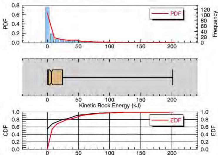
Figure C 4 – Barrier plot showing kinetic energy of modelled rockfall trajectories intersecting the proposed location of the rockfall fence on the hillslope to the true right of Brewery Creek (drawing 3209881-C001).
