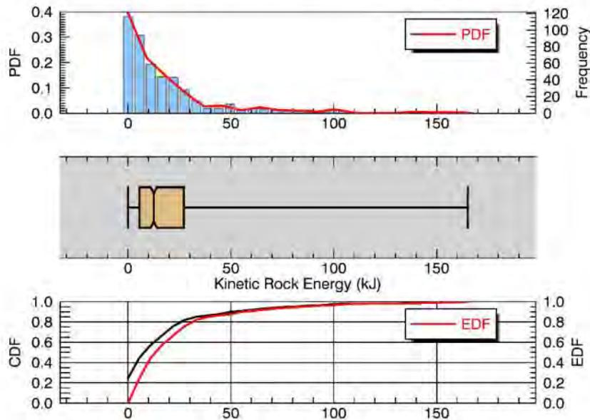
Figure C 2 - Barrier plot showing kinetic energy of modelled rockfall trajectories intersecting the proposed location of the rockfall fence on the hillslope to the true left of Brewery Creek (drawing 3209881-C001).
