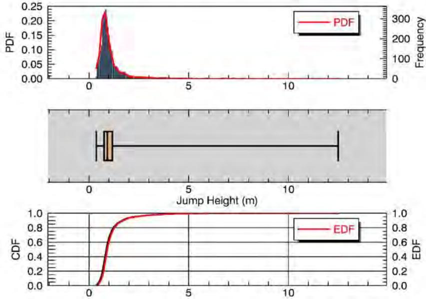
Figure C 7 - Barrier plot showing bounce heights of modelled rockfall trajectories intersecting the proposed location of the rockfall fence on the hillslope to the true left of Reavers Fan (drawing 3209881-C002).
