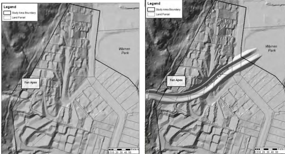
Comparison of the morphology of the existing Reavers Fan surface (left) and the proposed remedial channel (right).
