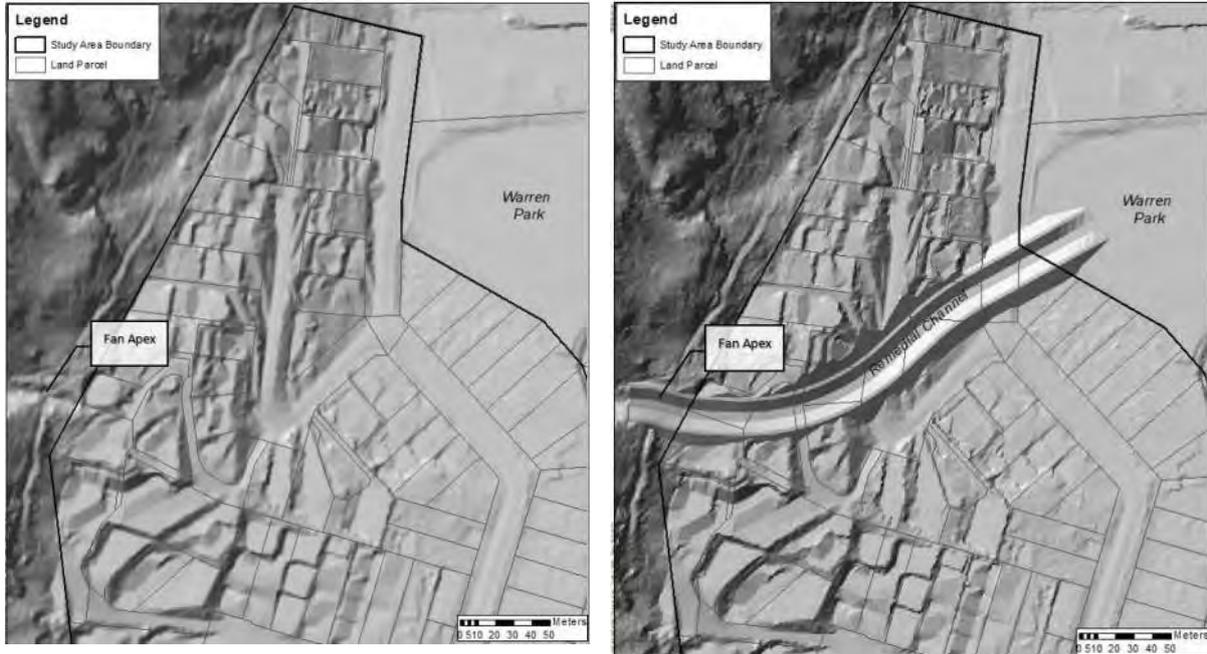
Figure 7 - Comparison of the morphology of the existing Reavers Fan surface (left) and the proposed remedial channel (right)
