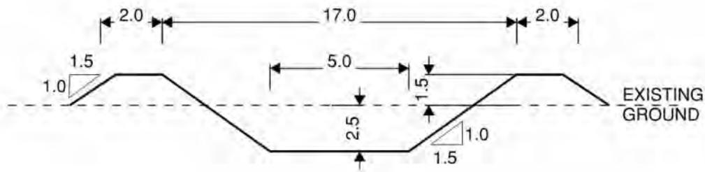
Figure A3 - Reavers Fan channel (new channel)
