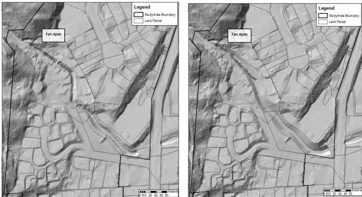
Figure 5 - Comparison of the morphology of the existing Brewery Creek channel (left) and the proposed modified channel (right).
