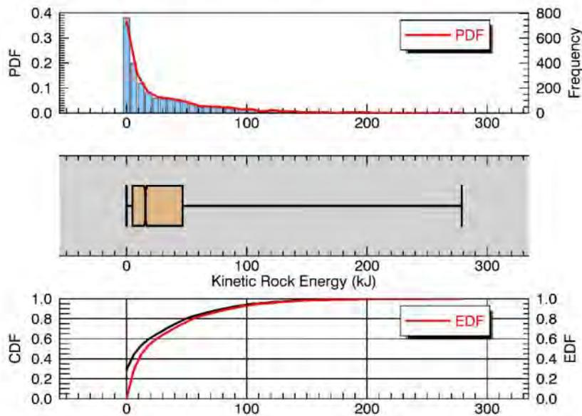
Figure C 6 - Barrier plot showing kinetic energy of modelled rockfall trajectories intersecting the proposed location of the rockfall fence on the hillslope to the true left of Reavers Fan (drawing 3209881-C002).
