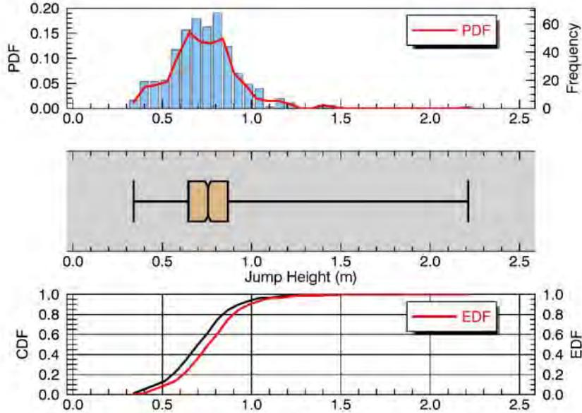
Figure C 1 - Barrier plot showing bounce heights of modelled rockfall trajectories intersecting the proposed location of the rockfall fence on the hillslope to the true left of Brewery Creek (drawing 3209881-C001).
