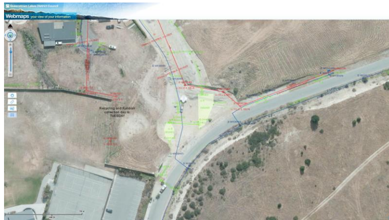
Figure 1 – Subject Sites and Existing Services (Storm Water Soakage Basins) Shown Green. Source – QLDC Website 05.03.15
